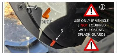
FIGURE J Remove INS2 inner fastener before installing into mount 4.
