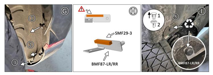
**FIGURE J** Place logo-side of mud flap facing rear of the vehicle against corresponding mounting points. Use 1.5SS & SMWASH to fasten points 1 - 3. Use SSLNUT and SMWASH for mount #4. Do not fully tighten.
