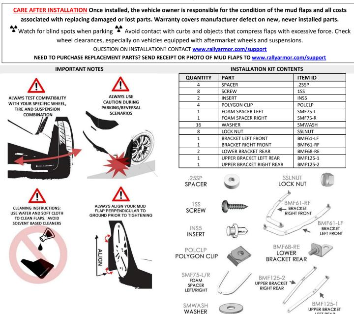
Recommended Tools Low-profile offset or ratcheting screw driver, 7/16<sup>th</sup> wrench, flathead screwdriver.
