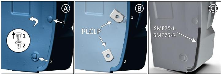
**FIGURE D/E** Place logo-side of mud flap facing rear of the vehicle against mounting points on liner. Position BMF61-LF/RF bracket against mounting points. Use SMWASH & SCREW 1SS to fasten points 1 & 2. Use a SMWASH & SSLNUT for points 3 & 4. Do not fully tighten.
