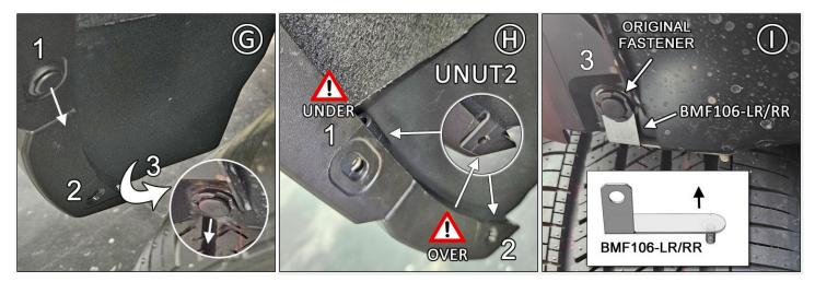
**IMAGE J** Place logo-side of flap facing rear bumper and against liner. Install SMWASH & 1SS into mounts 1 & 2 and SMWASH & SSLNUT into mount 3.
